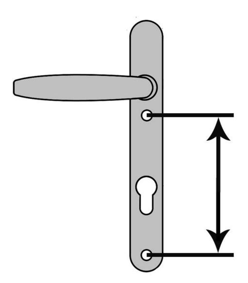
There are other measurements which you will find on door handle technical diagrams, however, these two measurements are the only ones required to ensure your replacement door handle fits and operates perfectly. All other measurements are there to outline the look and aesthetic of the uPVC door handle.
